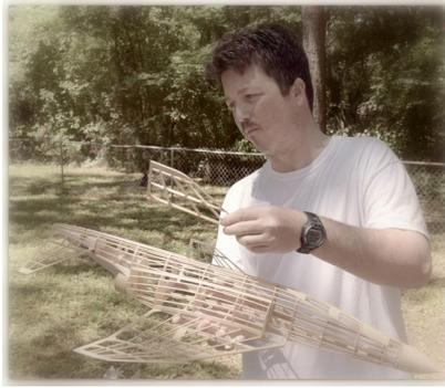
This concave area (above the exhaust ports) is copy paper with a balsa pattern printed on each side. Then I cut out the parts.
