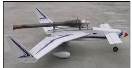
The extreme heat developed means that this engine needs a lot of air cooling and cannot stand static running on a test-bench for longer period than about 10 seconds. It must also be mounted outside the model to prevent burning damage to the structure. Due to the extreme noise and the high temperature involved, this engine is absolutely not recommended for beginners and should not be used near residential areas. ✈
