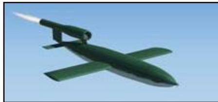
The Germans used this type of engine during WWII to power the well-known V-1 flying bomb. This power concept was eventually proven to be relatively inefficient, terribly noisy and also having a very short lifetime.
