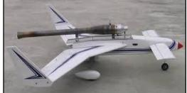
The extreme heat developed means that this engine needs a lot of air cooling and cannot stand static running on a test-bench for longer period than about 10 seconds. It must also be mounted outside the model to prevent burning damage to the structure. Due to the extreme noise and the high temperature involved, this engine is absolutely not recommended for beginners and should not be used near residential areas.  $\bigstar$
