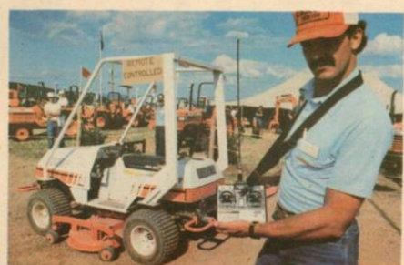
Dan Kilgas operates driverless mower using hand-held control panel. STEERS, STOPS AND STARTS BY REMOTE RADIO CONTROL
