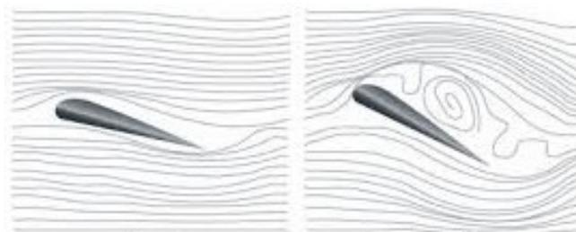
VGs introduce a high energy turbulent stream of air (a vortex) into the air flow causing a delay in separation of smooth air flow as the angle of attack increases.
