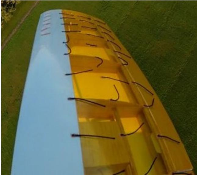
Notice how the tufts (showing airflow) are straight behind the VGs at the wing tip and in mixed directions on the rest of the wing.
