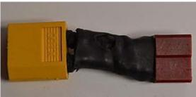
The use of adaptors like the one shown on the left gives you the ability to either use them on different setups or also for charge/discharge purpose.
