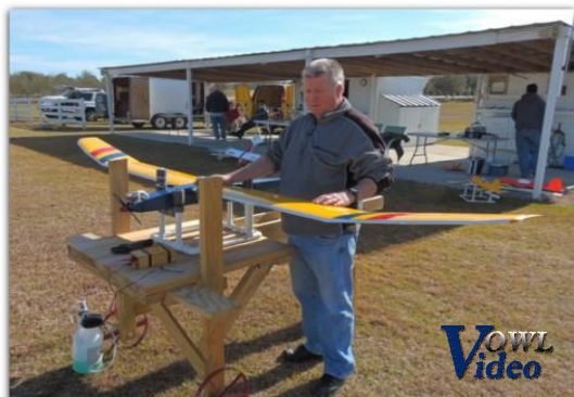
Mike's scratch-built glider patterned after the Spirit 100 with an OS .25 motor
