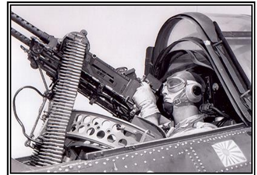
The ANM2 .30-cal. machine gun was designed for aircraft use and could fire 1,350 rounds per minute. Twin ANM2s were mounted in the rear seats of Dauntless dive-bombers. Marines used guns salvaged from them as the basis for the ground version of the "Stinger."
