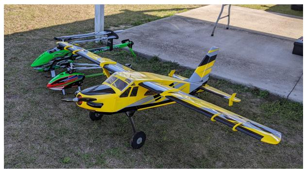
The vertical fins you see on the wings and the tail surfaces of the above aircraft, are called fences. They also appear on the wings the Mig-15 fighter. At some time in the future, I will present an article that explains these devices and how they can be helpful at low speeds.
